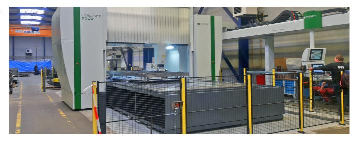
the concept of the UNIPORT4000 machine with a travelling bridge and stationary table. We have many CNC machines, but this was something completely new for us. The configuration simplifies the process of handling and machining weldments and sheet metal considerably."
