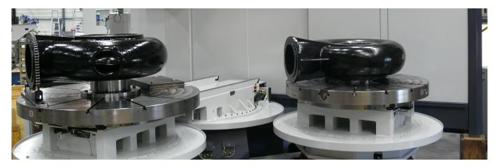
we produce have a diameter of around 1.3 metres and are over 2000 mm high. The components that we drill, turn and mill using our UNICOM6000 always consist of 1 to 3 individual pieces per set, in a variety of sizes. In most cases, they are made of cast iron."
