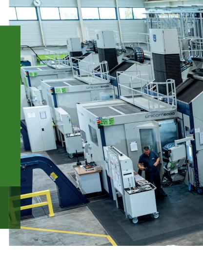
A total machining solution with three UNICOM6000 machines connected together via an FMS
