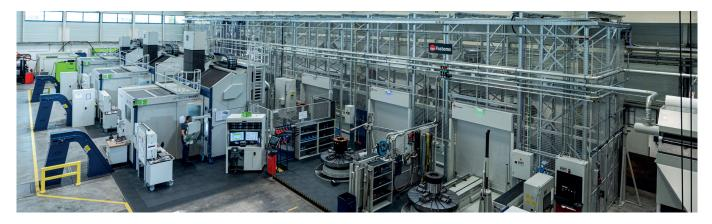
to a higher level, we decided to implement a total solution concept by linking three UNICOM6000 machines to a pallet-handling and warehousing system – a Fastems Flexible Manufacturing System (FMS). Of all suppliers we considered, Unisign was the one that came up with the most effective total solution." A one-off contract was issued for the solution as a whole (3x UNICOM with an FMS), and the lead role was entrusted to Unisign.
