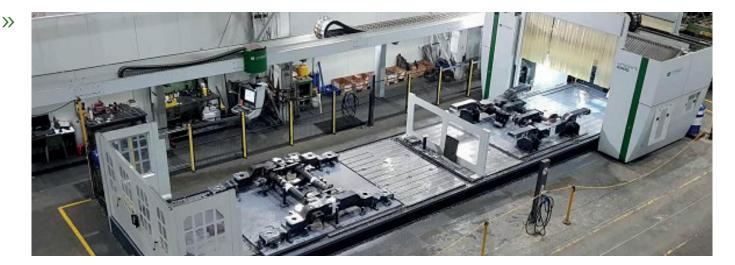
and it's very important for the profitability of the Bendigo site. It's located centrally in our workshop and forms the heart of our processes. We use it for machining railway bogies for about one full day a week. On the other six days of the week, we use the UNIPORT6000 for a variety of other machining work, such as gear casings."
