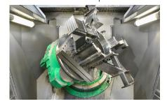
in Frauenfeld. When checking the Traoripoint (the pivot point of the turntable and swivel table), a dimensional inaccuracy was identified on the Z-axis. Clephas then corrected the Z-axis, before carrying out further measurements on the spindle in two temperature scenarios – hot and cold. The result? Both measurements were once again comfortably within the machine's specifications.
