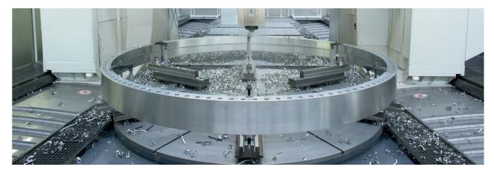
large component. Here at Brück, a component weighing 3 tonnes is classed as a small component. To give just one example: Wind turbines contain large rings that control the power transmission system. Rings of that type are the sort of products we typically produce."
